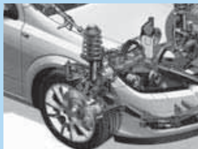
MacPherson strut front suspension.
