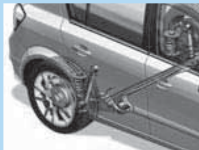
Lightweight torsion beam rear axle.
